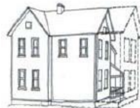
▪ Inappropriate: side two story addition
