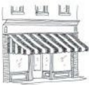
Awnings should reinforce openings, not cover features
