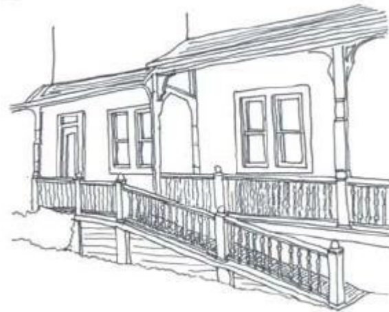
Ramp Addition to a porch
