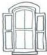
Does not fit arch
