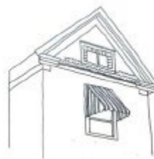
Awnings should fit the opening to which they are applied
